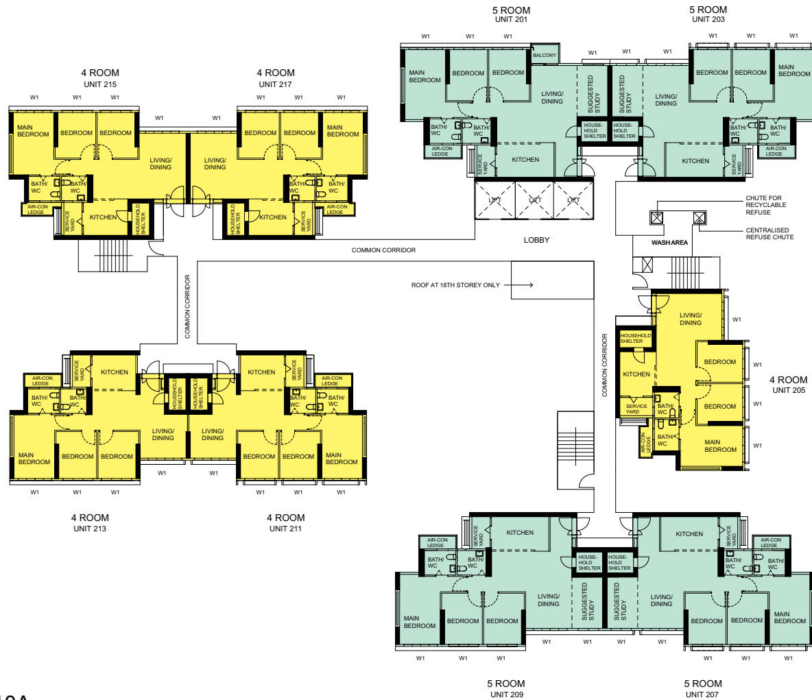
BLOCK 210A (18TH, 20TH, 22ND, 24TH AND 26TH STOREY FLOOR PLAN)
