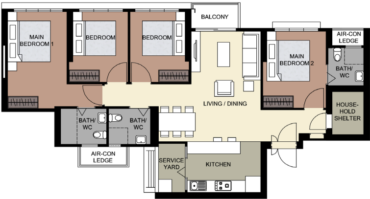
LAYOUT IDEAS FOR 3GEN FLAT APPROX. FLOOR AREA 123 sqm (Inclusive of Internal Floor Area of 118 sqm and Air-Con Ledges)
