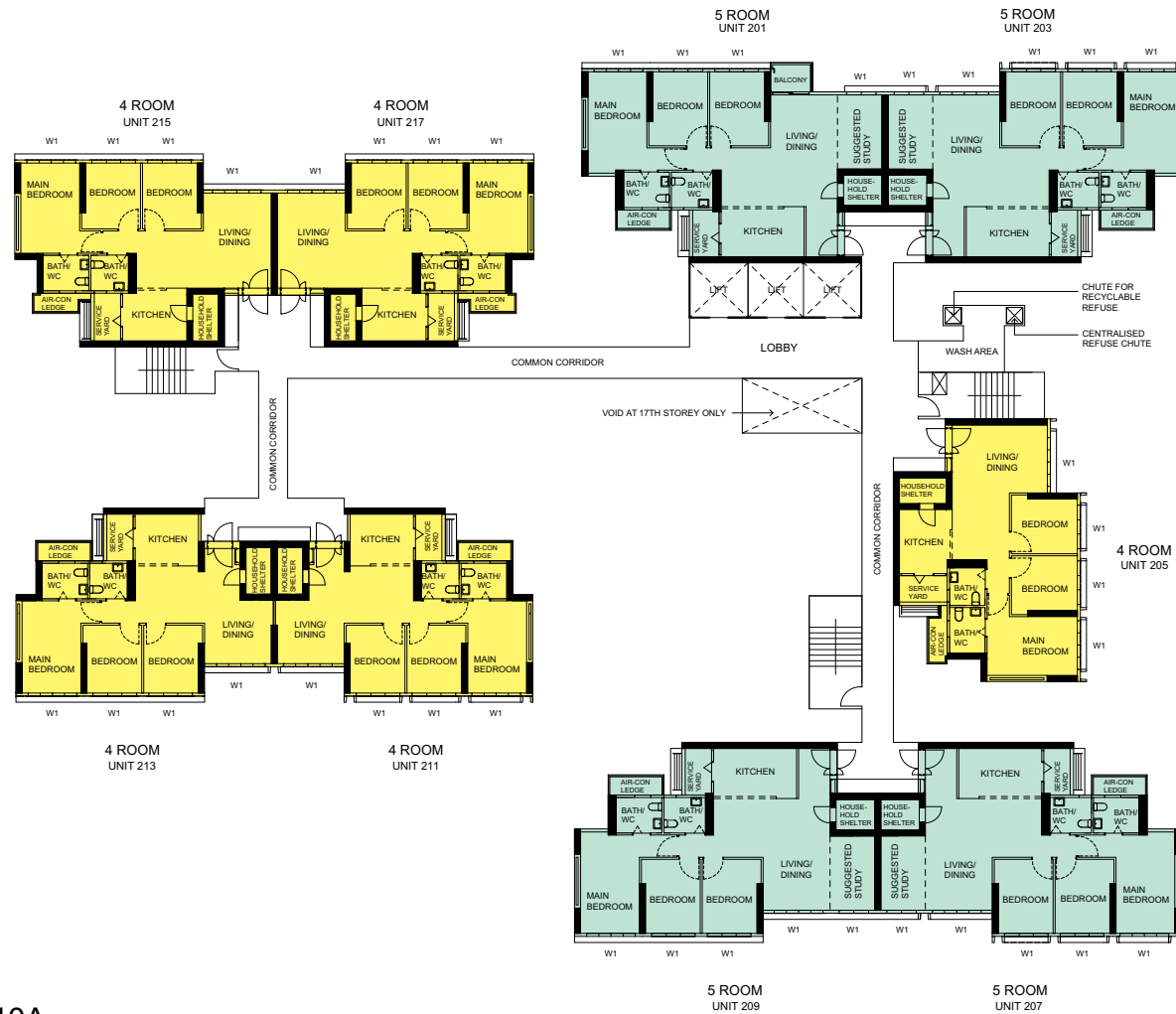
BLOCK 210A (17TH, 19TH, 21ST, 23RD, 25TH AND 27TH STOREY FLOOR PLAN)
